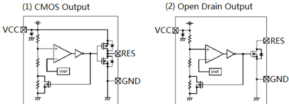
Figure 2 Block Diagram
