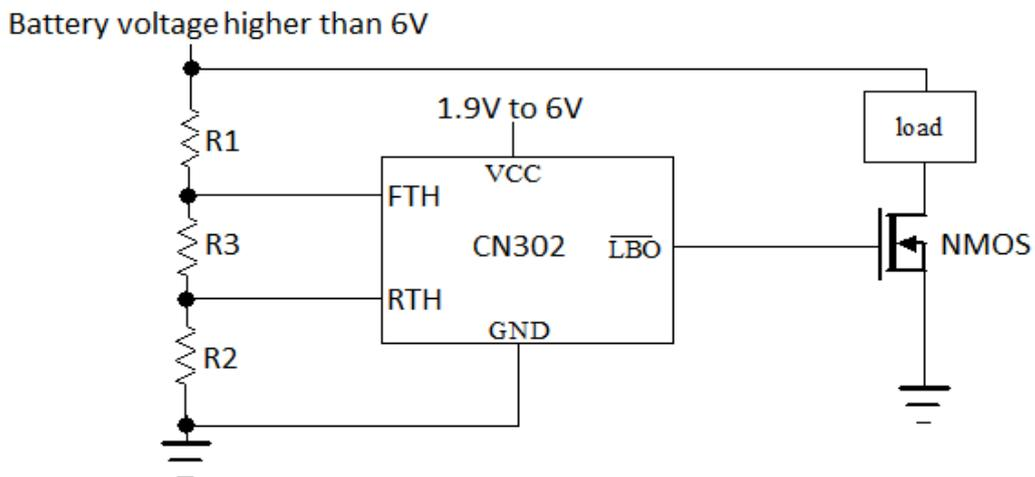
Figure 5  $V_{BAT} > 6V$ , CN302 controls N channel MOSFET
