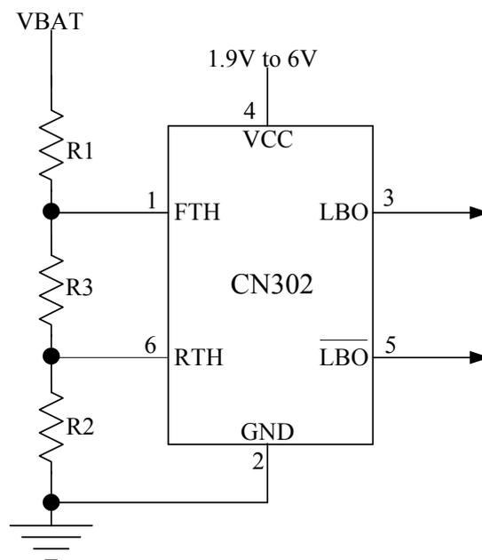
Figure 2 Monitoring Battery Voltage Higher Than 6V
