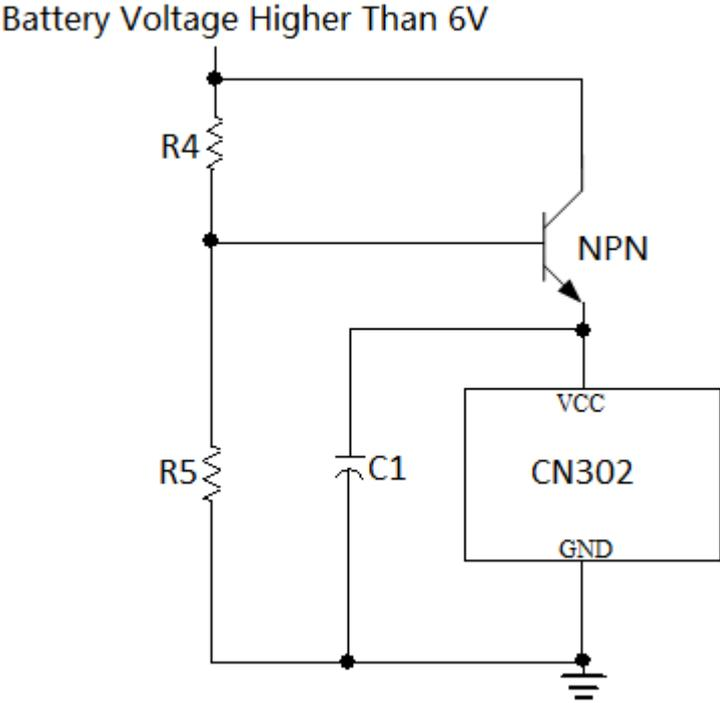
Figure 9 Power CN302 from a Resistor Divider
