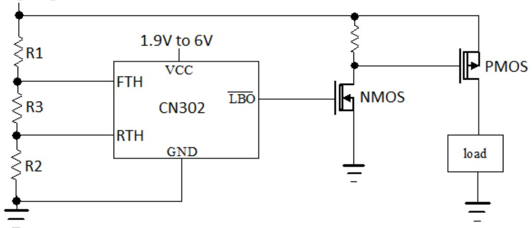
Figure 7  $V_{BAT} > 6V$ , CN302 controls P channel MOSFET
