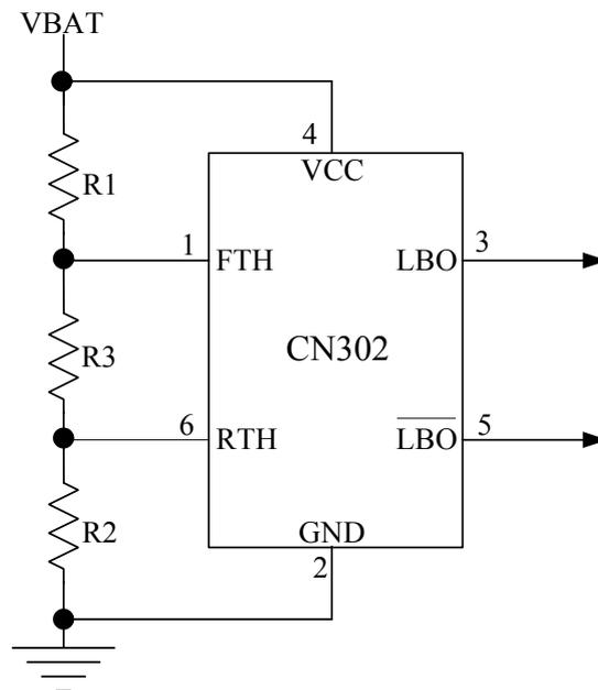
Figure 1 Monitoring Battery Voltage Lower Than 6V
