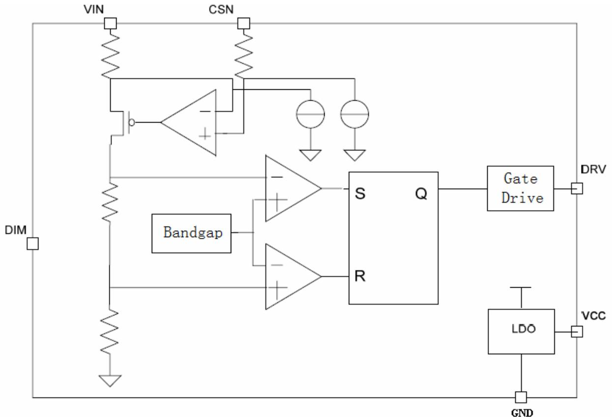
Figure 2 Block Diagram
