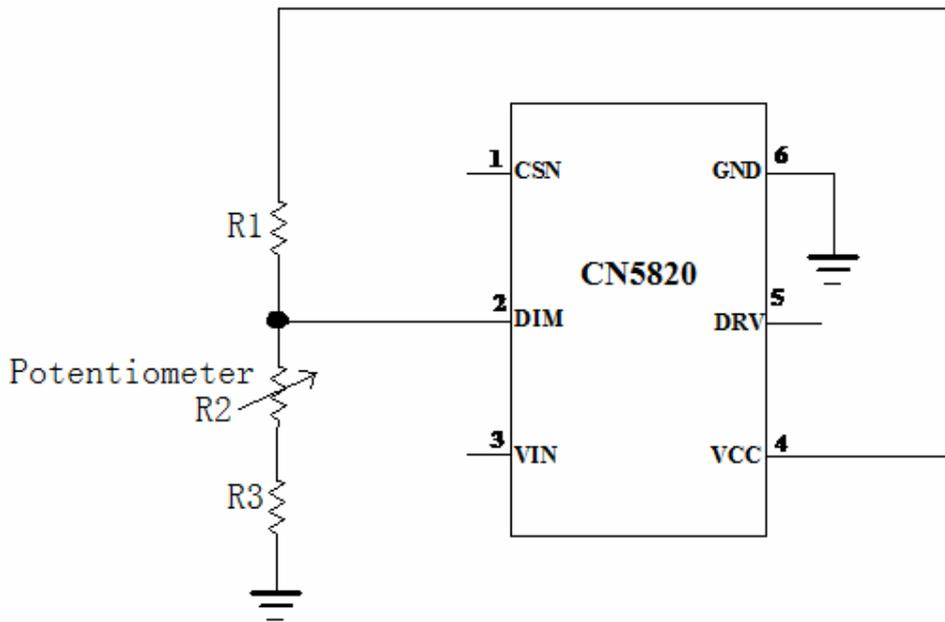
Figure 3 Analog Dimming by Using a Potentiometer
