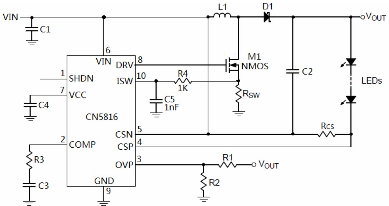
Figure 1 Typical Application Circuit of Buck-Boost Topology
