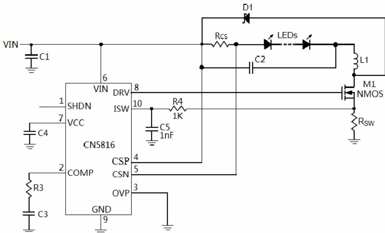
Figure 2 Typical Application Circuit of Buck Topology
